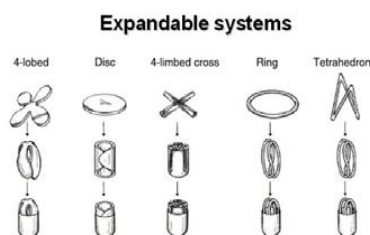
Fig.7. Different geometric forms of unfoldable systems (24)
